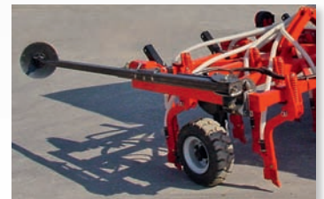
▲ -Hydraulic markers. Horizontal folding. / Traceurs hydrauliques. Pliage horizontale.
