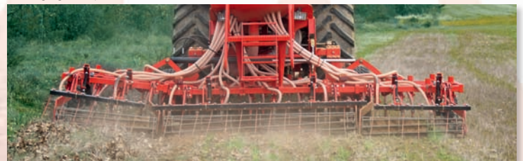
▲ -Independent wings are adapted to the field. / Ailes indépendantes adaptables au champ.
