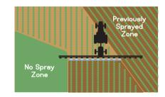
Individual GPS-guided boom section control gives you one of the most accurate and cost-efficient systems on the market, automatically avoiding no-spray zones and previously sprayed areas.
