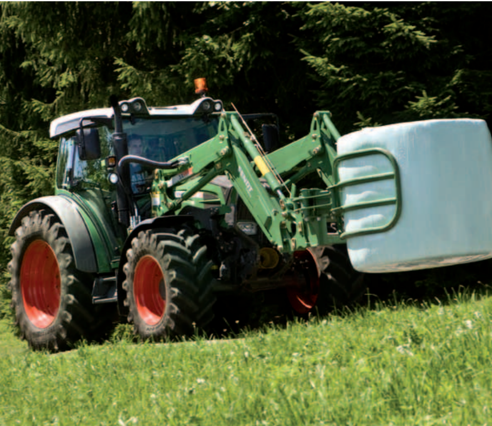
Mechanical self-levelling – compact design through Z-bar linkage
