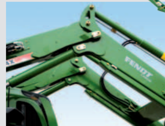
Mechanical self-levelling – compact design through Z-bar linkage
