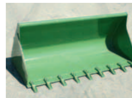
The heavy-duty bucket is available in the widths 1600 mm (0.512 m³ flush volume) and 2100 mm (0.672 m³ flush volume)
