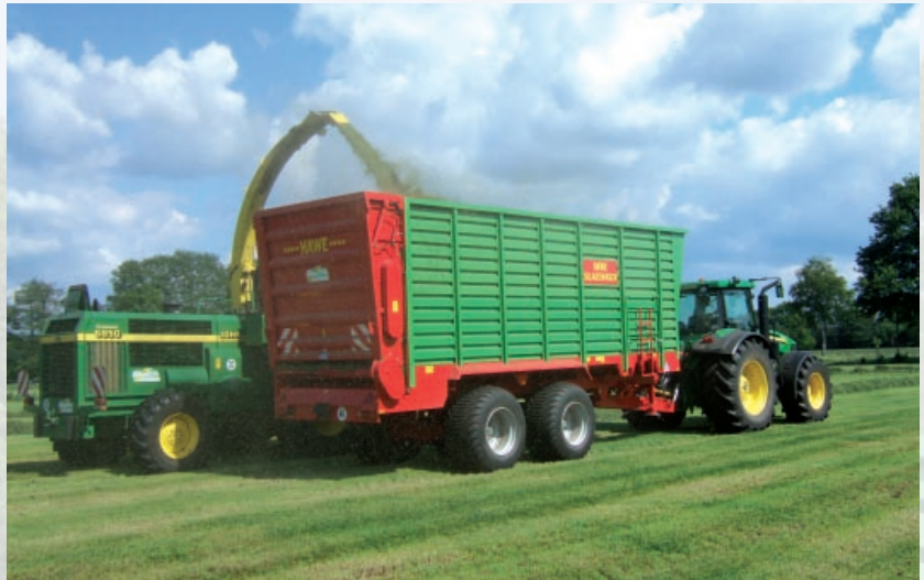
SLW 45 with hydraulic chassis and lower hitch with a licensed gross weight of 23 tons
