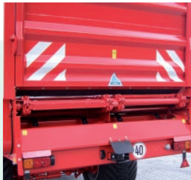
SLW 45 with steel bottom and heavy scraper floor chain (14 x 50 mm) located above
