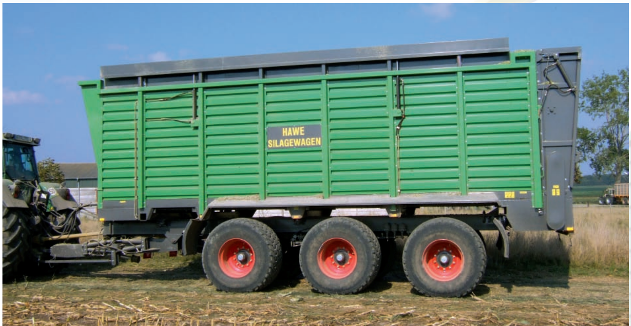
SLW 50 tridem, hydraulic chassis with lifting axle, restricted steering mechanism, tyre equipment Cargo X Bib 710/50 R 26.5 and hydraulic side-wall lifting
