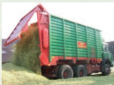
A container with a capacity of 35 cubic metres for attachment on the truck. The capacity can be extended up to 45 cubic metres with 4-axle trucks
