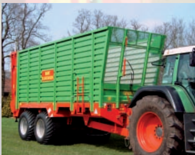
SLW 40 with 800/45 x 26.5 tyres, hydraulically movable front wall providing a good view of the container interior
