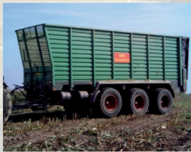
HAWE SLW 50 tridem as exchange system, lower hitch with ball-shaped coupling K 80, restricted steering, air-suspended chassis with automatic axle-lifting facility, Michelin Cargo X Bib 710/50 R 26.5 tyres
