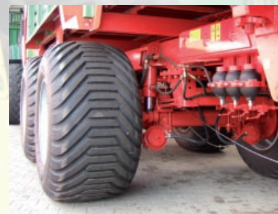
SLW 45 with twist-lock system and hydraulic spring suspension for the chassis (optional)
