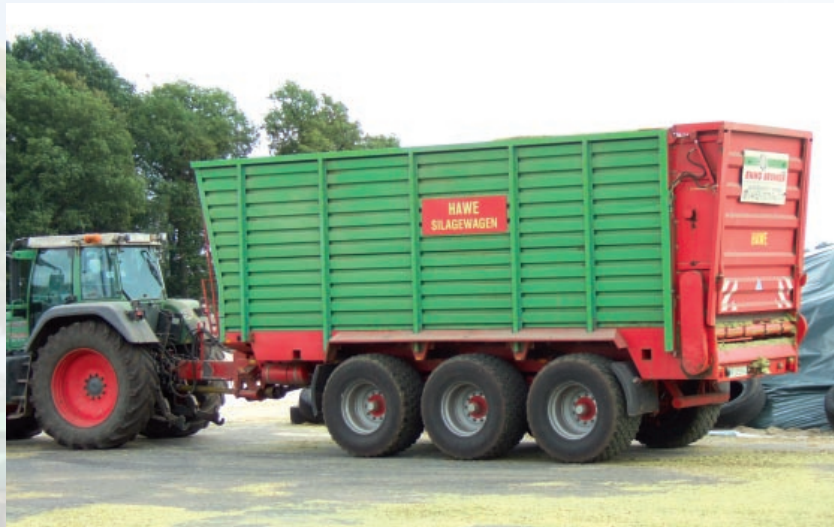
SLW 45 tridem with Michelin Cargo X Bib 600/55 R 26.5 tyres and an upper hitch as exchange system
