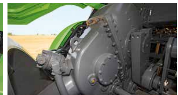
A new high-capacity gearbox is used in the XD baler. Overall, the XD gearbox is 35% heavier than the standard model and can therefore generate even more compression pressure.
