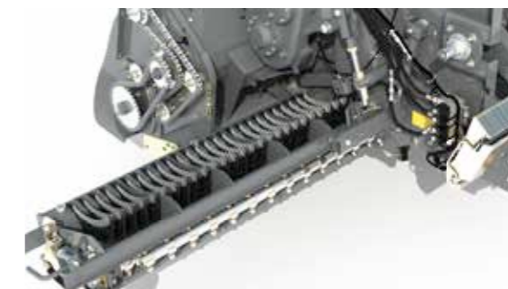
The lowered knife drawer can be pulled out on the left side of the machine to change knives.
