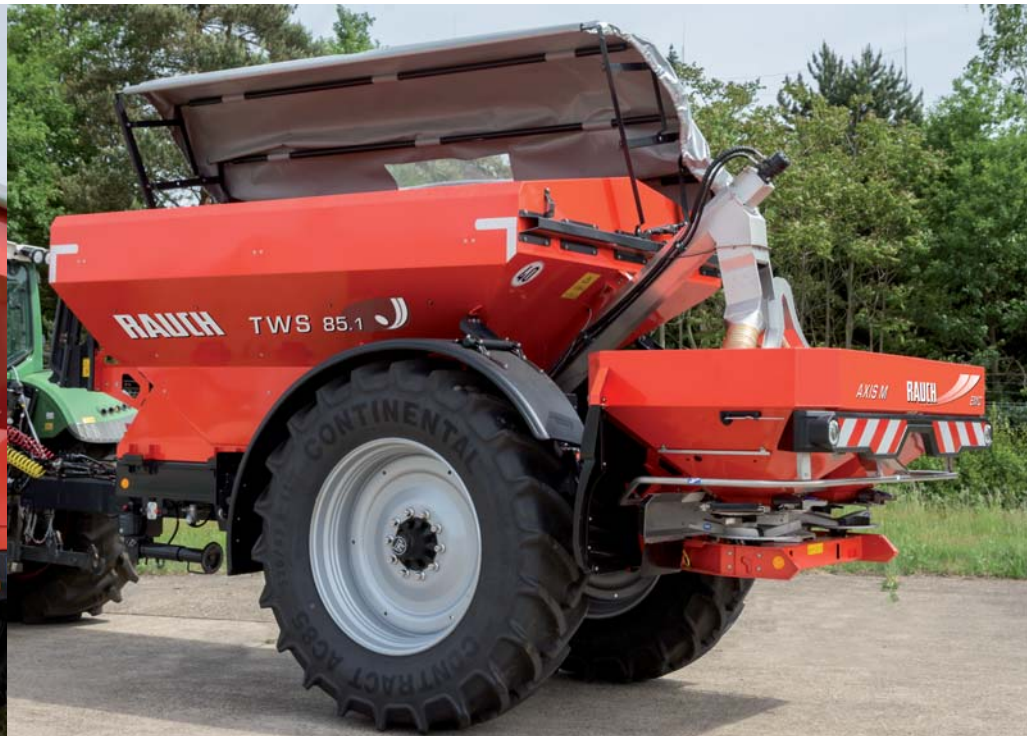
The TWS hopper cover and the central metering slide are hydraulically remote-controlled for high operating comfort.
